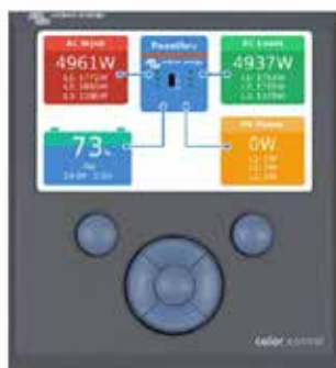
Color Control GX, showing a PV application
