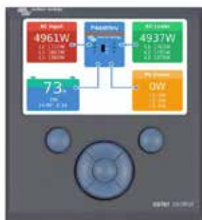
Color Control GX, showing a PV application
